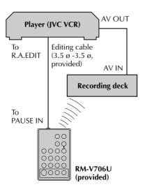
Using the RM-V706U remote control, it is also possible to perform deck-to-deck Random Assemble Editing. The playback deck must be an R.A. Edit-capable JVC VCR. The recording deck can be...
